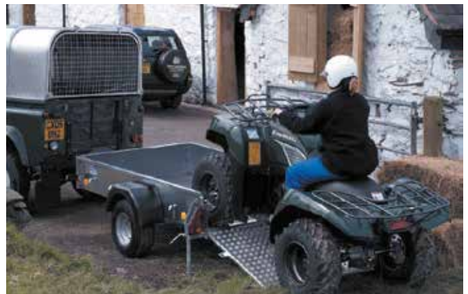
P7e ramp model with optional propstands
